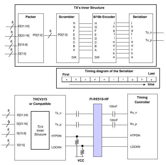
notes: 1. The LCD module uses a 100 nF capacitor on positive and negative lines of each receiver input.
